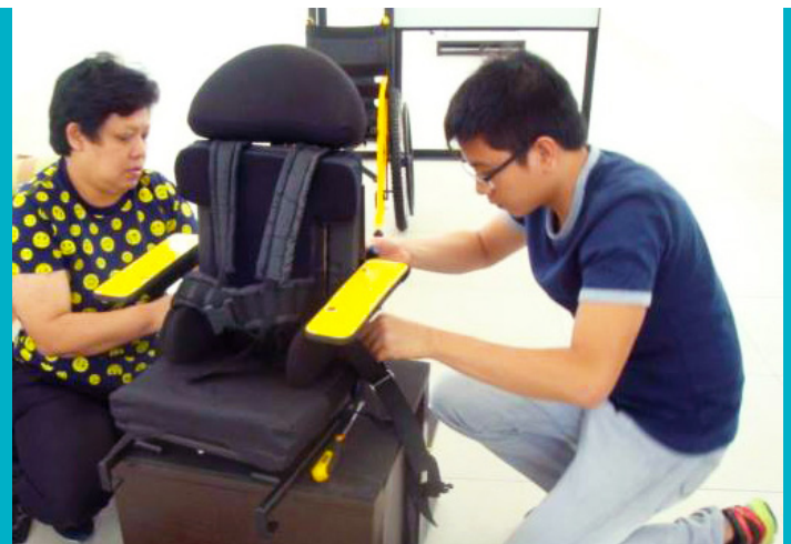
Attaching cushions and safety straps for a child-customized wheelchair seat. Photos from the Philippine Society of Wheelchair Professionals https://www.facebook.com/pg/WheelchairTrainingPSWP/photos/
